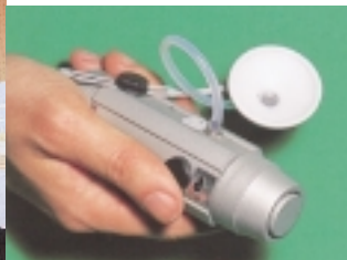
Fig. 2 Pitch controlled artificial larynx
