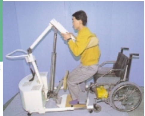
Fig. 3 Transfer aid using a Metal-Hydride actuator
