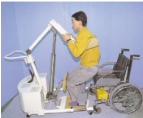
Transfer aid using a metal-hydride actuator.
