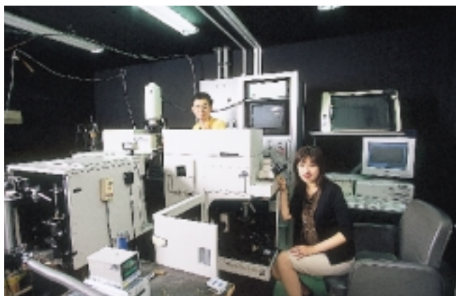
Raman scattering system for the study of proton dynamics in the hydrogen-bonded material.
