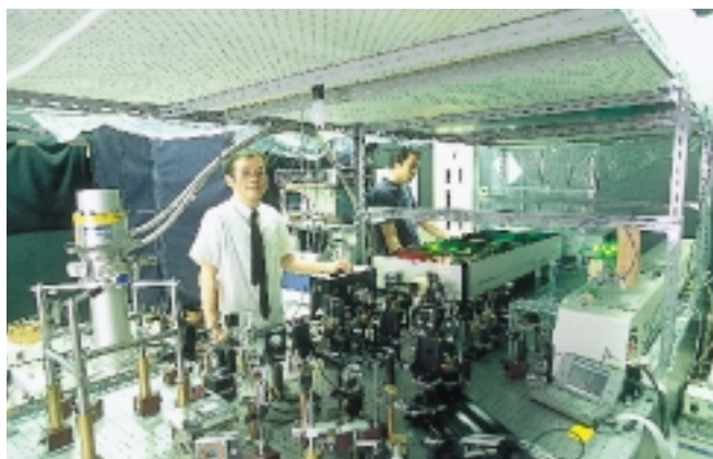
Femtosecond Q-sw mode-locked Ti:sapphire laser system for the study of ultrafast dynamics.
