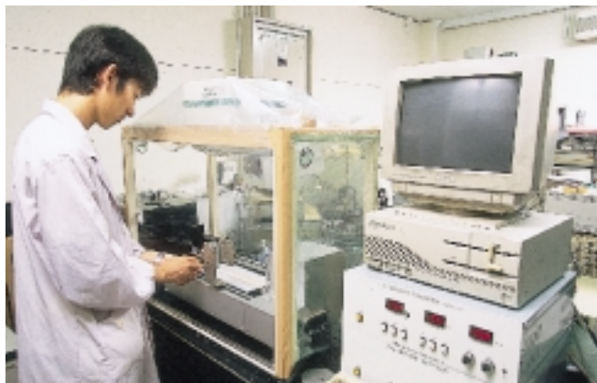
Fabrication of a clay-organic molecule hybrid LB film.
