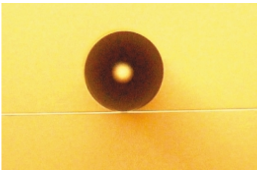
A microsphere with a stem contacted with a tapered fiber.
