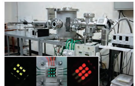
Chemical vapor deposition system and OLED emission
