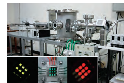
Chemical vapor deposition system and OLED emission.
