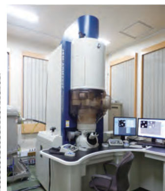
CsSTEM (Right) and an atomic resolution STEM image of SrTiO 3 (Left).
