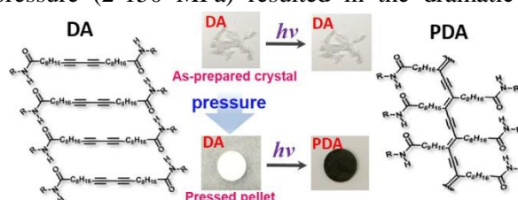
Fig. 1. Pressure-induced transition of DA from light-inert state to photopolymerable state forming PDA.
