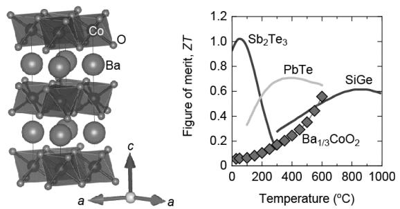
**FIG. 2 |** (Left) Schematic crystal structure of  $\text{Ba}_{1/3}\text{CoO}_2$ . (Right) Temperature dependence of the  $ZT$  of the  $\text{Ba}_{1/3}\text{CoO}_2$  epitaxial film in the in-plane direction. Comparison against commercially available p-type thermoelectric materials. The  $ZT$  of the  $\text{Ba}_{1/3}\text{CoO}_2$  epitaxial film at 600 °C is comparable to that of p-type PbTe and p-type SiGe.
