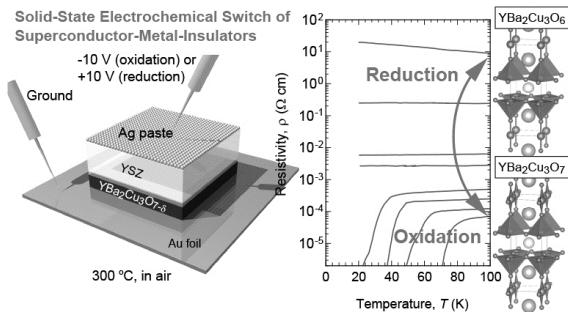
**FIG. 1 |** (Left) Schematic device structure of a solid-state electrochemical switch of superconductor-metal-insulators. The device is operated at 300 °C in air by applying  $\pm 10$  V. (Right) Temperature dependence of electrical resistivity for  $\text{YBa}_2\text{Cu}_3\text{O}_{7-\delta}$  films. The  $\delta$  values were modulated electrochemically.
