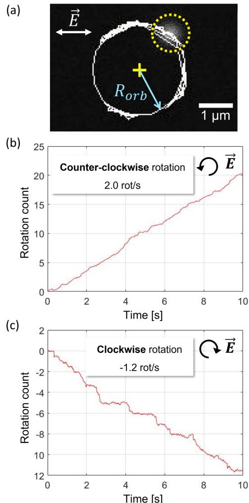
図 1 (a) Circular trajectory (orbit radius  $R_{\text{orb}}$ ) of a  $\text{VO}_2$  particle trapped by a linearly-polarized, focused Gaussian laser beam. The particle is located inside the dashed circle. (b),(c) Angular position of the  $\text{VO}_2$  particle trapped using a circularly-polarized, focused Gaussian laser beam: (b) Left-handed circular polarization, (c) Right-handed circular polarization.
