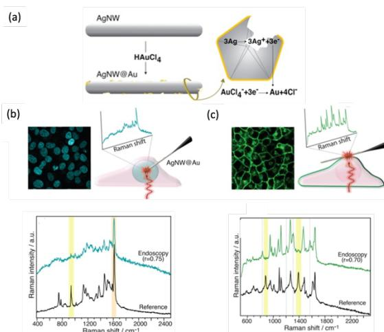
図2 Chemical and morphological changes induced by the galvanic replacement reaction (GRR) and yielding gold-etched AgNWs (Au-etched AgNW). (Adapted from Anal. Chem. 2021, 93, 5037–5045)
