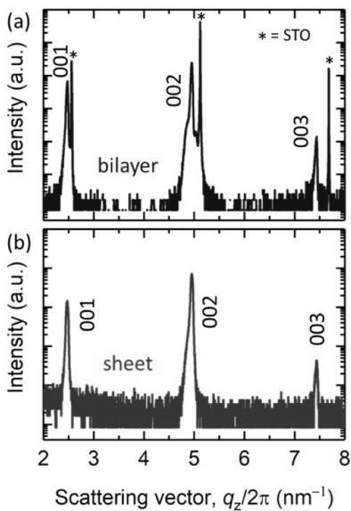
**FIG. 4** | Out-of-plane XRD patterns of the (a) LSSO/SAO bilayer film and (b) LSSO sheet.
