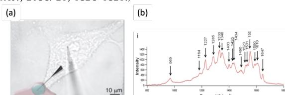
図1(a) Transmission image of an AgNW endoscopy probe upon insertion into the cell nucleus of a single HeLa cell. Inset: An endoscopy experiment schematic. (Adapted from Anal. Chem. 2021, 93, 5037–5045) (b) An example of the remote excitation SERS spectrum taken from the nucleus of a single live HeLa cell. (Adapted from Adv. Mater., 2014, 26, 5124–5128.)
