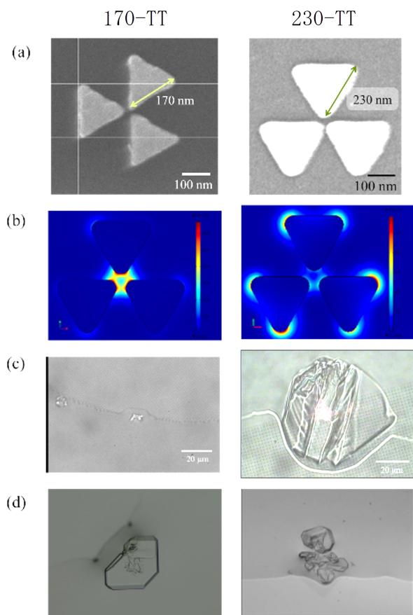
図2 (a) SEM images of 170 nm (left) and 230 nm (right) triangular trimers. (b) Simulation results showing the enhanced electric field of 170-TT and 230-TT excited by a 1064 nm-wavelength light. (c) Transmission images showing the size of the induced crystal with 170-TT and 230-TT (d) Transmission images showing the numbers of crystal induced by 170-TT and 230-TT.
