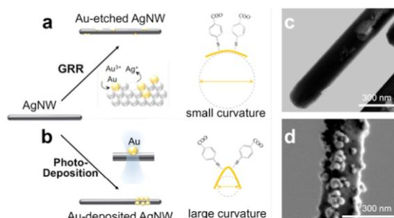
図3 Schematic illustration of the fabrication of a Au-etched AgNW via GRR (a) and a Au-dep AgNW via photodeposition (b). STEM and SEM images of an Au-etched AgNW (c) and a Au-dep AgNW (d), respectively. (adapted from ACS Appl. Nano Mater. 2021, 4, 9886–9894)
