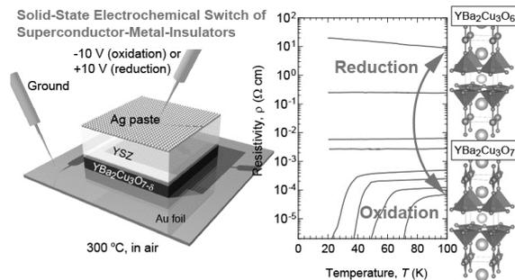
**FIG. 1** | (Left) Schematic device structure of a solid-state electrochemical switch of superconductor-metal-insulators. The device is operated at 300 °C in air by applying  $\pm 10$  V. (Right) Temperature dependence of electrical resistivity for  $YBa_2Cu_3O_{7-\delta}$  films. The  $\delta$  values were modulated electrochemically.
