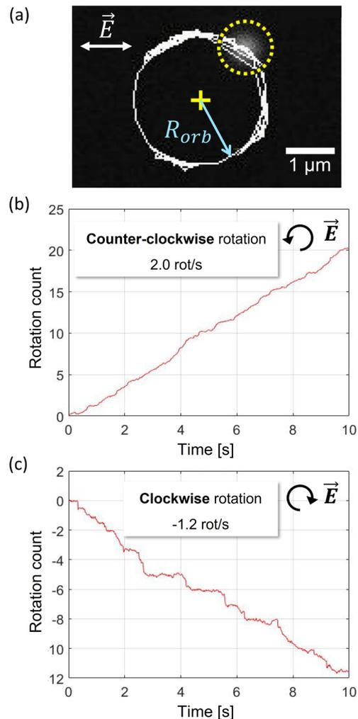
図1 (a) Circular trajectory (orbit radius  $R_{orb}$ ) of a  $\text{VO}_2$  particle trapped by a linearly-polarized, focused Gaussian laser beam. The particle is located inside the dashed circle. (b),(c) Angular position of the  $\text{VO}_2$  particle trapped using a circularly-polarized, focused Gaussian laser beam: (b) Left-handed circular polarization, (c) Right-handed circular polarization.
