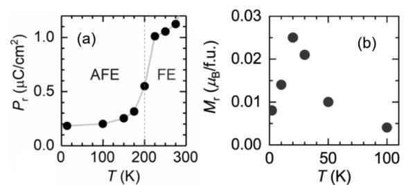
FIG. 3 | (a) Remnant polarization of  $k$ - $\text{DyFeO}_3$  film and (b) remnant magnetization of  $k$ - $\text{ErFeO}_3$  film as a function of temperature.
