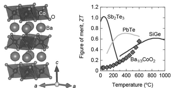
**FIG. 2** | (Left) Schematic crystal structure of  $Ba_{1/3}CoO_2$ . (Right) Temperature dependence of the  $ZT$  of the  $Ba_{1/3}CoO_2$  epitaxial film in the in-plane direction. Comparison against commercially available p-type thermoelectric materials. The  $ZT$  of the  $Ba_{1/3}CoO_2$  epitaxial film at 600 °C is comparable to that of p-type PbTe and p-type SiGe.
