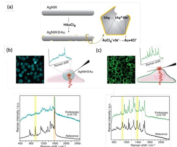
図2 Chemical and morphological changes induced by the galvanic replacement reaction (GRR) and yielding gold-etched AgNWs (Au-etched AgNW). (Adapted from Anal. Chem. 2021, 93, 5037-5045)
